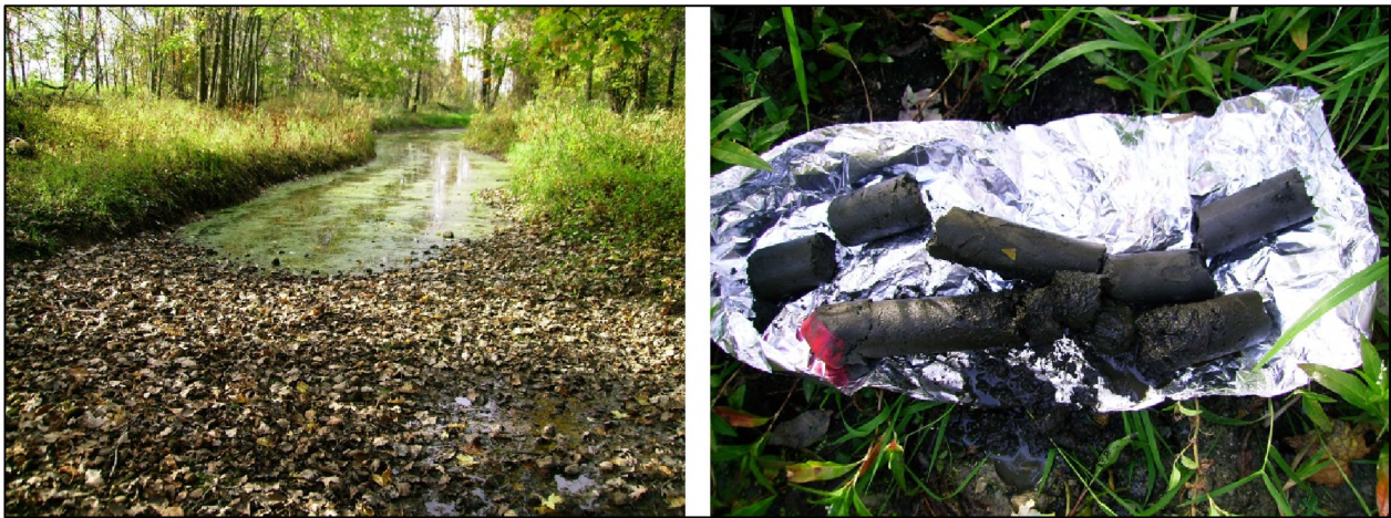
Figure 4: The left photo shows the northern end of the rocky channel section indicated by the blue pushpin in Figure 3. From here the swampy, low-flow portion of the river extends to the north and west as shown in Figures 1 and 2. The photo on the right shows a core sample taken upstream from the rocky area in standing water. The core went down approximately 1 m and did not hit rocks.
